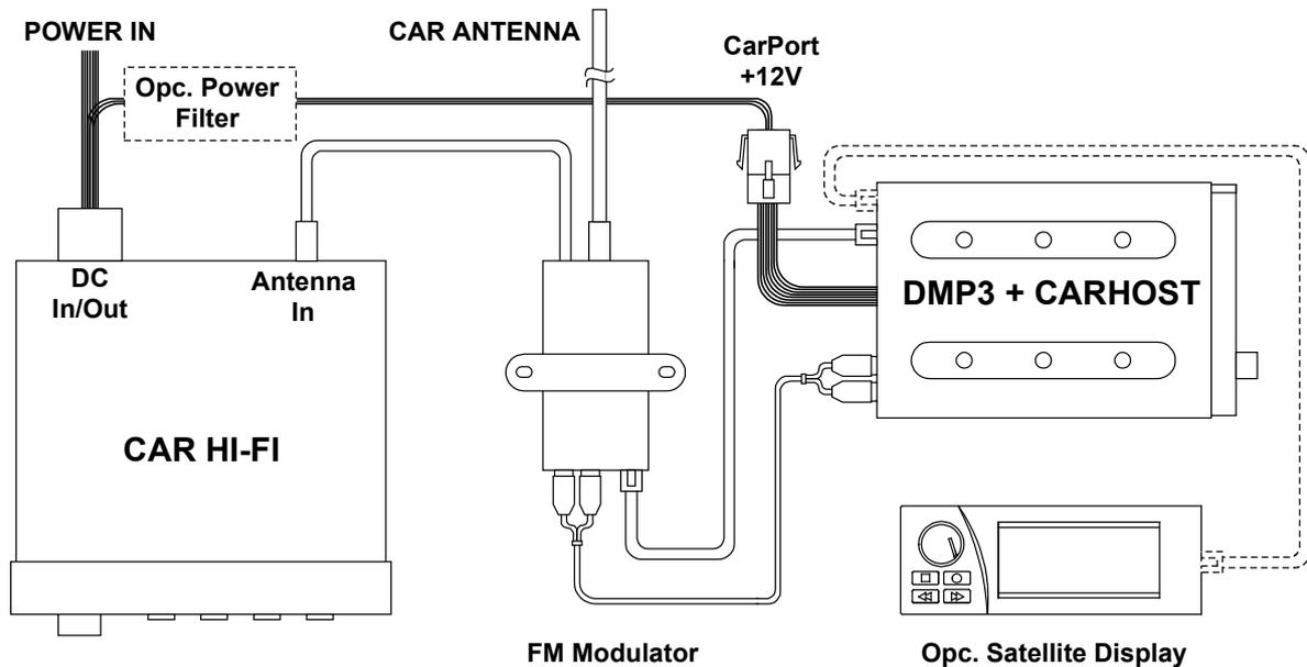
Because of the above mentioned specifications, the best place to install the **FM Modulator** is somewhere near the car radio, for example behind it, or in the glove compartment. If the enclosed cable is too short, use an extension cable available in car shops
