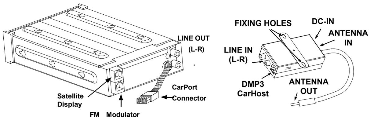
The **FM Modulator** is connected to the **DMP3** through the CarHost frame. Power supply and data communication needed for controlling the frequency happens through the RJ11 6/6 cable, which needs to be connected to the appropriate output of the CarHost. Sound signal can be connected from the line output using shielded RCA cable. The order of making the connections is irrelevant.
